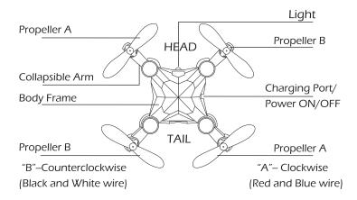
Please note that all propellers must be installed in the correct orientation.(Pay attention to the letter "A" or "B" printed on each propeller when installing.)
