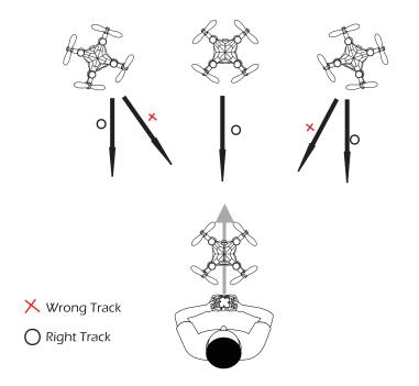
With a press of the One Key Return button, the drone will return along the parallel direction where the tail of the drone pointed to when the drone was paired.
