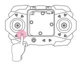
© Press One Key Take-off button, the drone will take off automatically. Or push throttle(left) joystick up slowly to take off and ascend the drone.
