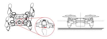
② First, slide the "Power Switch" button right to turn on the drone. Then, place the drone on flat and level surface with the head facing forward and the tail facing towards the pilot.
