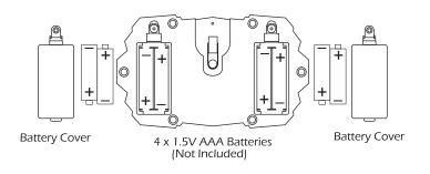
Note: Always pay close attention to battery polarity when inserting any batteries to make sure they are fitted correctly.
