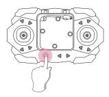
③ Then, trun on the Transmitter. One second later, one beep will be heard and the drone's indicator lights will start flashing and then turn solid, indicating that the drone and the transmitter have been paired successfully and automatically.
