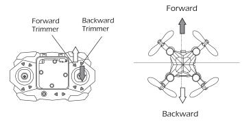
**®** Forward/ Backward Sideward Fly Trim: When the drone drifts forward, press the backward trimmer button to rebalance the drone; if the drone drifts backward, press the forward trimmer button to rebalance the drone.
