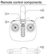
1 Power switch 2 Left joystick (press and hold for trimming adjustments and release when finished) 3 Phone holder 4 Right joystick (short press to toggle between
