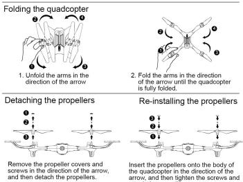
Note: The propellers are labelled "A/B". Ensure that each propeller is inserted in the corresponding position on the arms, and then tighten the screw.and ther tighten the screws and attach the propeller covers.
