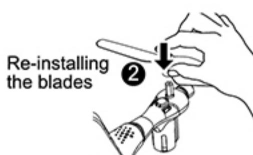
\* A labeled blades fit on the A labeled motors. Blabeled blades fit on the B labeled motors. Use the screws to tighten the blades. Refer to the image.
