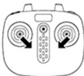
Push the left and right joysticks downwards in a V shape for 2 seconds.
