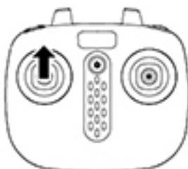
Move the left stick (throttle) fully up, after let it come back to the middle and the motors will start spinning.
