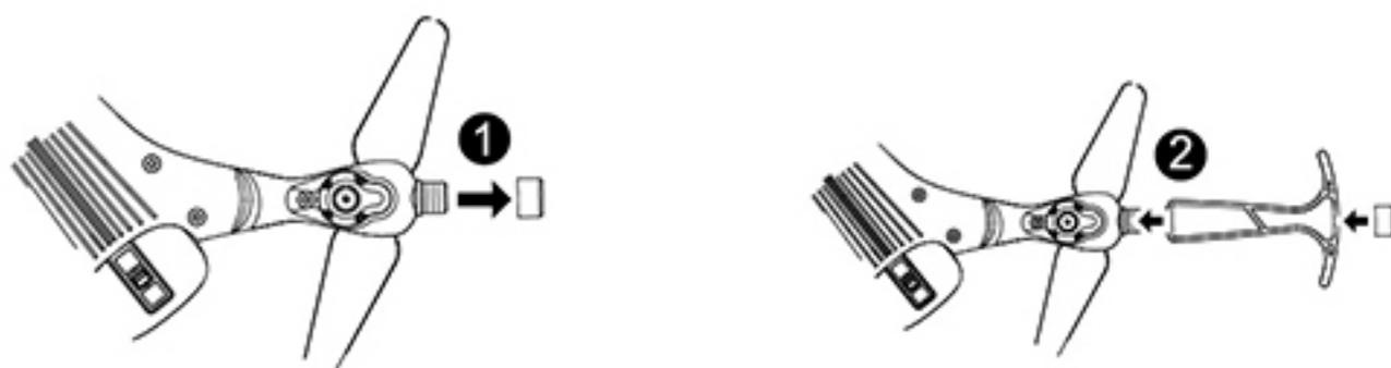
1. Remove the light cover on the drone.
