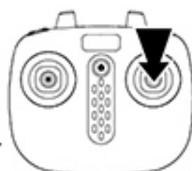
Briefly press the right joystick to switch between high and low speed mode.
