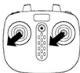
When the drone encounters a direct impact with foreign objects in the headless mode, if there is an occurrence of deviation of the defined direction, it is only required to push both the left and right joysticks to the bottom left corners simultaneously after placing the flying direction of the drone in the correction position. When the led light indicator of the drone is in a long "ON" mode after slowly flashing for 3 seconds, it indicates the calibration is complete.
