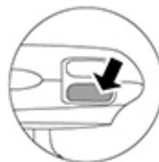
Press the take-off/landing button to make the aircraft land automatically and switch off.
