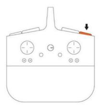
Press the orange FLIGHT button to lift off. Drone will elevate off of the ground and level off into a hover.
