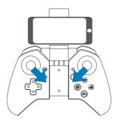
**Unlocking the motors**: Push two levers down to 45° as picture shows, until four rotor blades start rotating.
