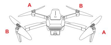
Connect each propeller to its corresponding motor shaft, either position 'A/B', then lock the propeller to the motor shaft with a screw.
