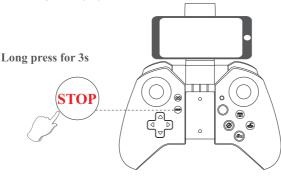
As shown above, long press the Emergency Stop button for 3 seconds, the motor will stop immediately.
