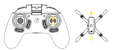
To fly the drone to the left or the right, push the Direction stick cautiously to the left or the right.
