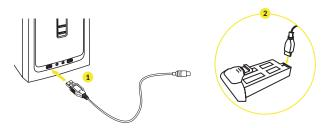
Connect the Micro USB Charging Cable to a USB port 1 and the battery of the drone. 2 A green LED light on the battery will indicate it is charging. When the battery is fully charged, the LED light on the battery turns off. It takes about 30 minutes to recharge a discharged battery.
