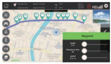
Waypoint parameter setting Click the waypoint to be set, and the setting menu will pop up. Hold down the ball and slide to modify the parameters.
