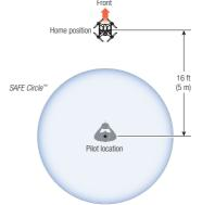
CAUTION: When the home location is set, the quadcopter must be approximately 16 feet (5 meters) from where the pilot will stand during flight, pointing away from the pilot. If the aircraft is pointed in any other direction, the SAFE Circle™ feature will not function as expected and may result in personal injury or damage to property. Once the aircraft's motors are started, do not change your position.
